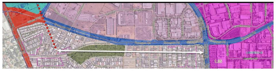
2.1 Upgrading to a 2-lane dual carriageway ('boulevard treatment'): on ultimate 4-lane alignment with a 13m raised median from Windsor Road to Hartman Drive before 2031. Intersection with existing Gnangara Road (Wanneroo Rd to Klaraborg Dr) to remain until MRWA grade separation. (assumed no MRRG Rehab prior).
