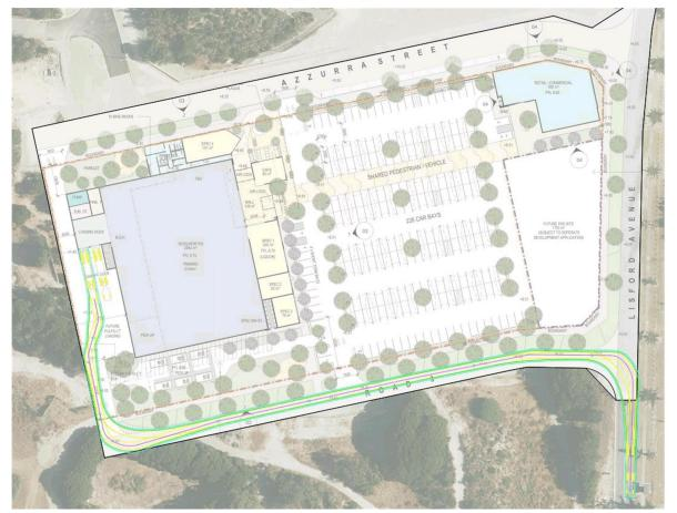
Figure 3-8 Swept Paths for a 19m Semi-trailer (Loading Dock 2 IN)
