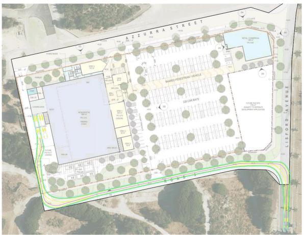
Figure 3-7 Swept Paths for a 19m Semi-trailer (Loading Dock 1 OUT)
