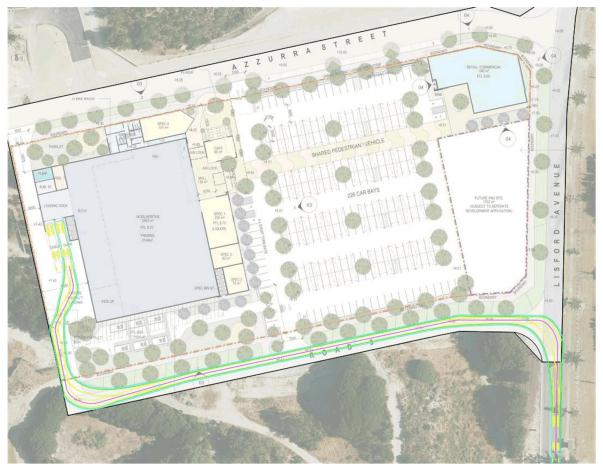
Figure 3-9 Swept Paths for a 19m Semi-trailer (Loading Dock 2 OUT)
