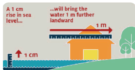
Figure 5.27 – Schematic representing the horizontal erosion allowance from projected vertical sea level rise – a factor of 100 (Coast Adapt 2017)
