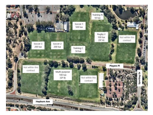
The above aerial plan shows the filed with the lighting levels post the completion of the works under Tender Number 22090.
