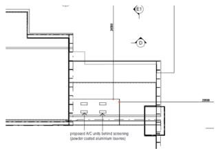
FIGURE 02 - LOCATION OF AIR CONDITIONING CONDENSING UNITS
