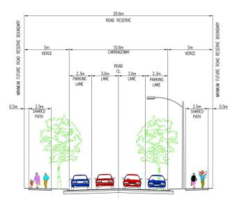
FIGURE 13: CROSS SECTION OF ACCESS STREETS B
