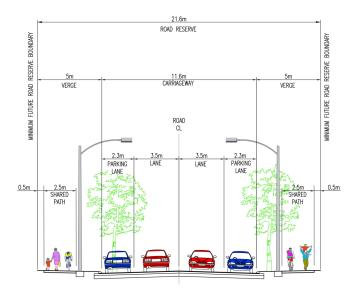
FIGURE 9: CROSS SECTION OF NEIGHBOURHOOD CONNECTOR B
