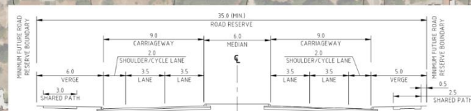
TYPICAL ROAD CROSS SECTION 1 CH 100 to CH 1500
