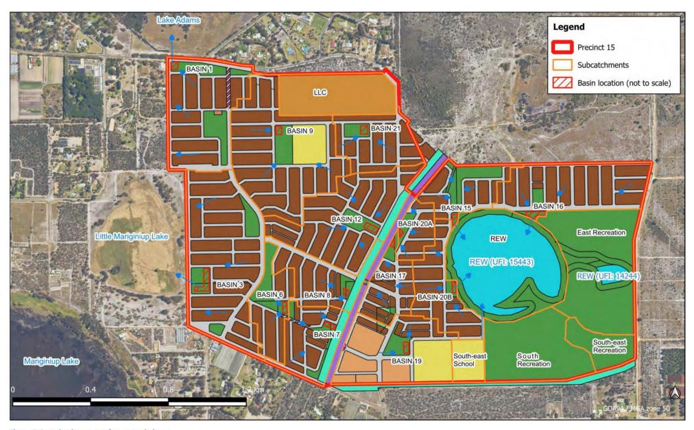
Figure 15: Post-development surface water drainage
